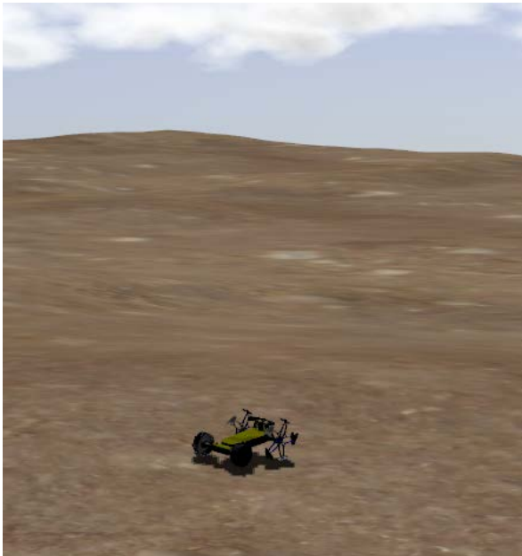
Figure 7. Scout rover on the Martian surface in Gazebo, built from HiRISE data.
