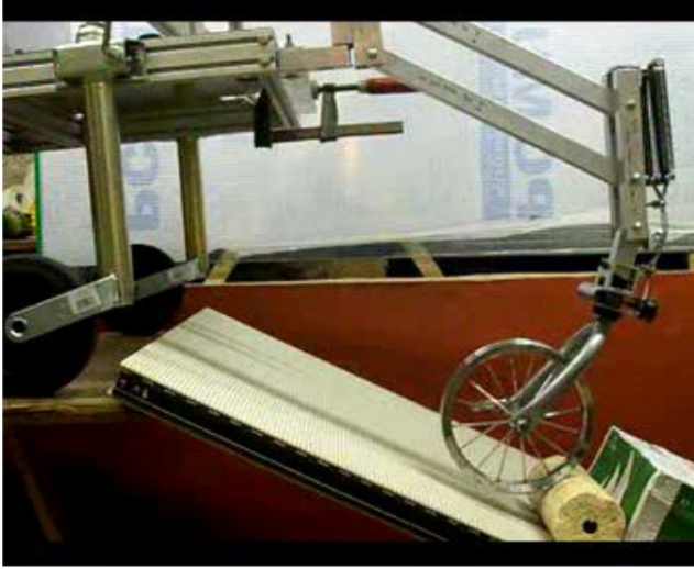
Figure 9. Mechanical mock-up of WB undergoing functional testing (LSG, V. Eder)
