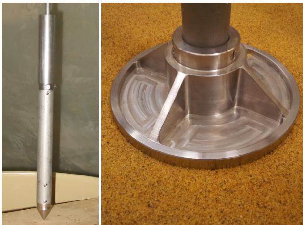
Figure 6. Early Dynamic Cone Penetrometer (left) and Dynamic Plate (right) instruments with a manual dropped mass. The DP sensor end (right) replaces the DCP cone shown in the left image to share a common impact mechanism.
