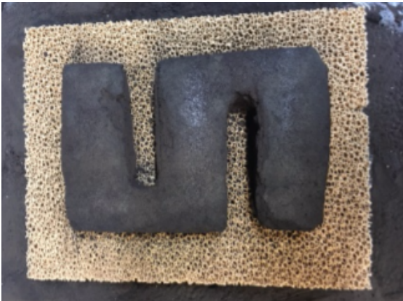
Figure 4: 3D-printed S-shape part with the Ambient system inside solar simulator. Image: DLR/Regolight consortium.
