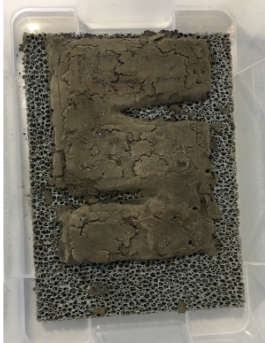
Figure 12: S-shaped part printed with the Mobile Printing Head. Image: Space Applications Services/Regolight consortium.
