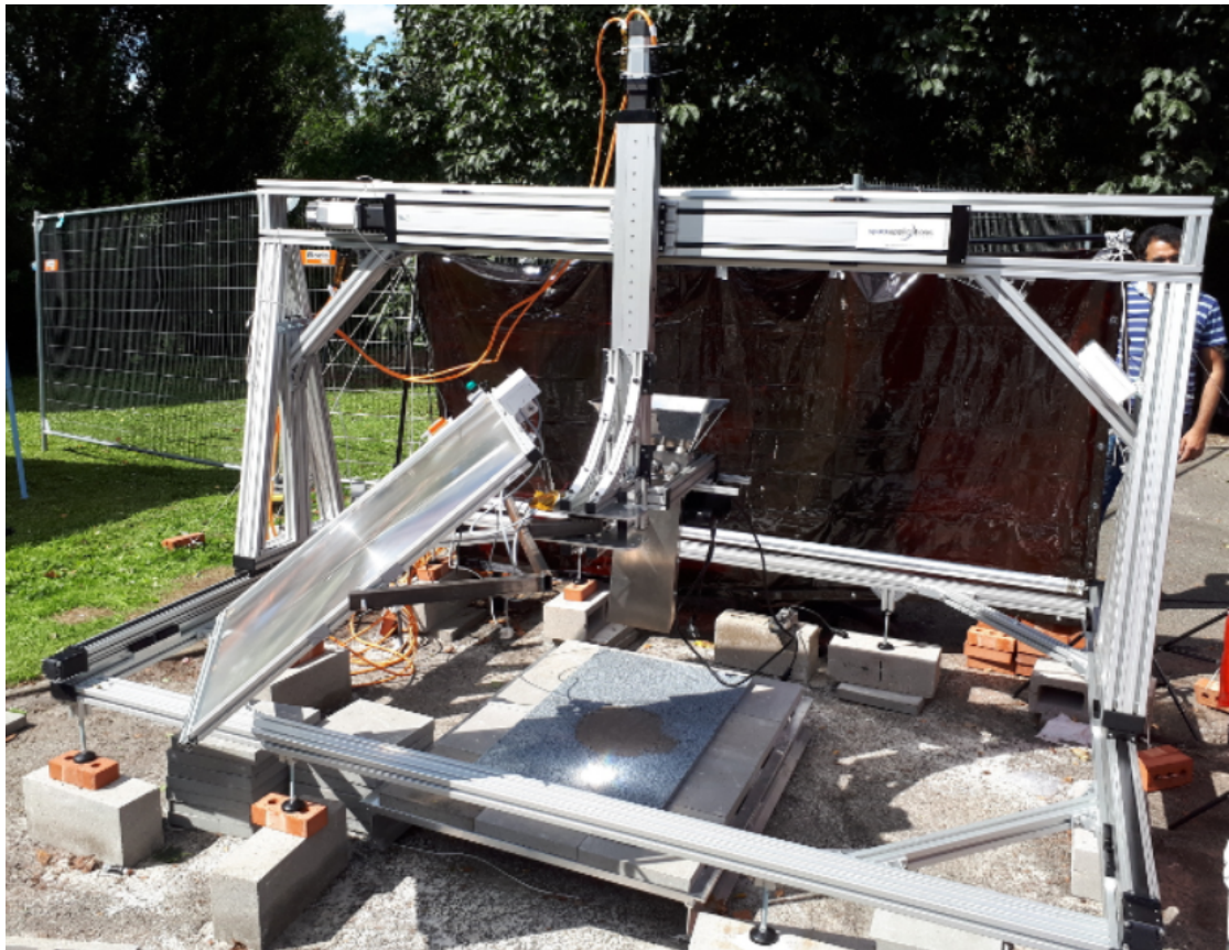
Figure 13: Gantry-based Mobile Printing Head assembled and in operation. Image: Space Applications Services/Regolight consortium.
