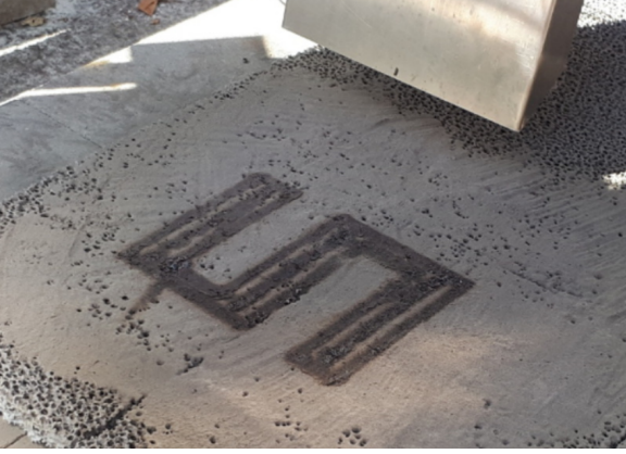
Figure 8: Sintered lines made on the JSC-2A lunar regolith simulant during preliminary testing. Image: Space Applications Services/Regolight consortium.
