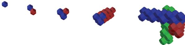
Figure 21: Assembly of larger brick units based on dodecahedral cells, credit: RegoLight consortium, visualisation: Bollinger Grohmann, 2018
