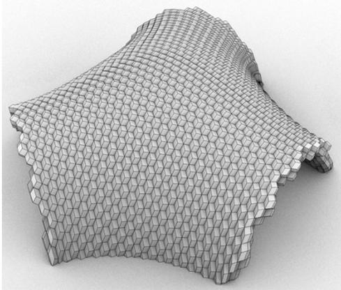
Figure 24: Shape derived from hanging model for compression only stress state under deadweight; credit: RegoLight consortium, visualization: LIQUIFER Systems Group, 2017
