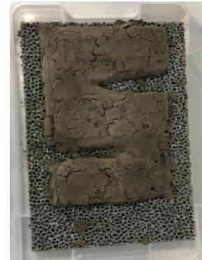
Figure 15: Printed Specimen, credit: RegoLight consortium, photo: Space Applications Services
