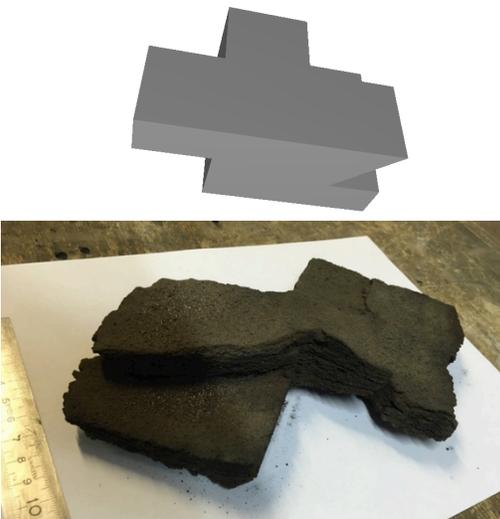
Figure 3: Computer designed complex object (top) and actual sintered part (bottom), credit: RegoLight consortium, photo: DLR
