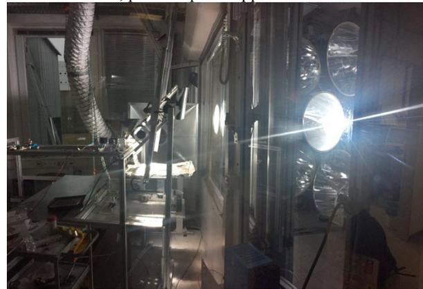
Figure 8: Solar sintering campaign in operational state, credit: RegoLight consortium, photo: LIQUIFER Systems Group
