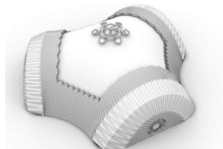
Figure 19: Lunar habitat with protection shield made up of RegoLight interlocking elements, credit: RegoLight consortium, visualisation: LIQUIFER Systems Group, 2018
