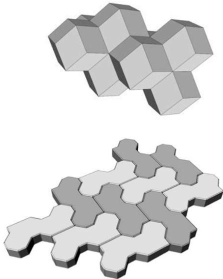
Figure 17: Top: Rhombic Dodecahedron selected for the mobile printing campaign. Bottom: Surface battlement structure selected for vacuum printing campaign, credit: RegoLight consortium, visualisation: LIQUIFER Systems Group 2017
