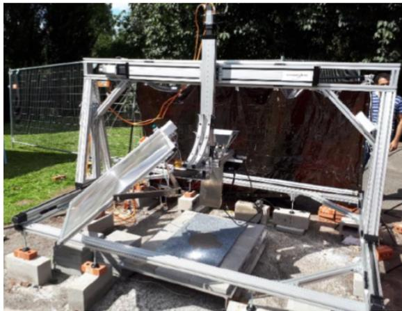
Figure 9: Mobile printing head as implemented, credit: RegoLight consortium, photo: Space Applications Services
