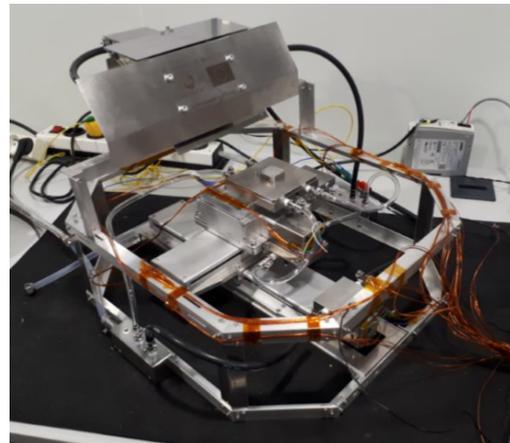
Fig. 10: Completed setup for the vacuum experiment (thermal covers not shown), credit: RegoLight consortium, photo: Space Applications Services
