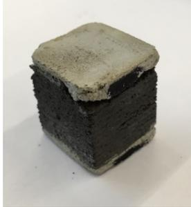
Figure 12: One 20 mm x 20 mm x 20 mm of sintered lunar regolith covered with gypsum - typical compression test sample, credit: RegoLight consortium, photo: DLR
