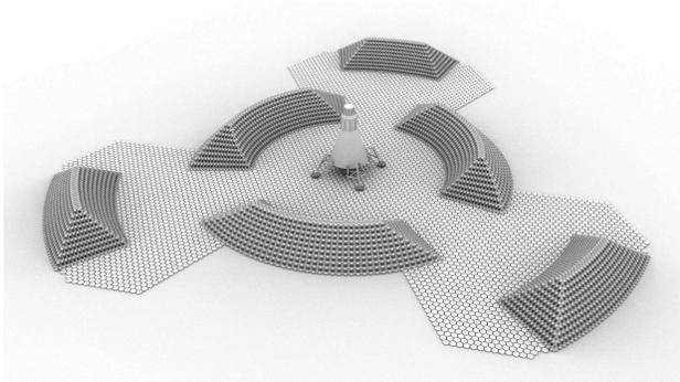
Figure 20: Launch pad with dust protection shield and flat terrain made made up of RegoLight interlocking elements, credit: RegoLight consortium, visualisation: LIQUIFER Systems Group, 2018
