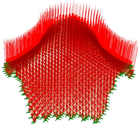
Figure 25: Finite Element model consisting of beam elements with loads and support conditions, credit: RegoLight consortium, visualisation: Bollinger Grohmann, 2018
