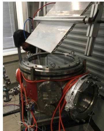
Figure 11: The chamber with the 3D printer installed under the solar furnace mirror, credit: RegoLight consortium, photo: DLR
