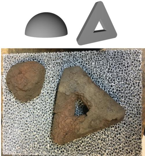
Figure 2: Computer designed half-sphere and triangle (top) and actual solar 3D printed parts (bottom). Support size 21 cm x 30 cm, credit: RegoLight consortium, photo: DLR
