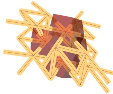
Figure 23: Idealization of contact conditions between the tetrahedral brick elements using beams using compression-only conditions, credit: RegoLight consortium, visualisation: Bollinger Grohmann, 2018
