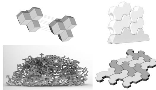
Figure 18: Geometries of interlocking building elements for 3D formfitting stackable top left, 2.5-dimensional elements top right, 3D randomly packed aggregates bottom left, 2-dimensional interlocking elements bottom right, credit: RegoLight consortium, visualisation: LIQUIFER Systems Group
