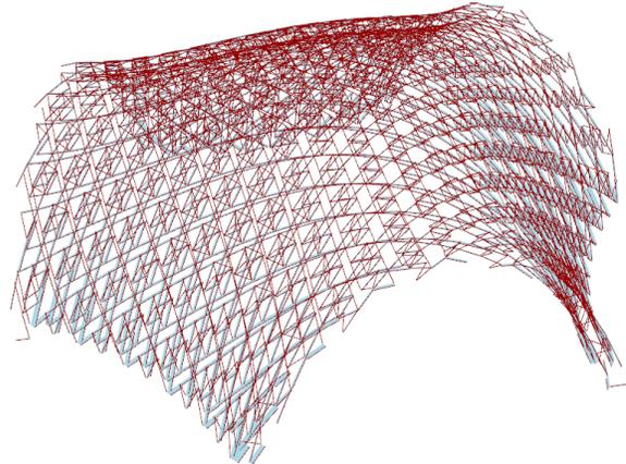
Figure 26: Compressive normal forces in final structure with contact elements under tension removed. The stability of the remaining structure proves the viability of assembling structures from element with compression-only connections., credit: RegoLight consortium, visualisation: Bollinger Grohmann, 2018
