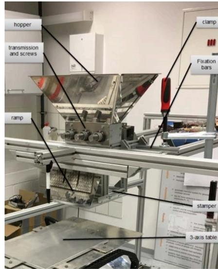
Figure 7: 3-axis table setup with feeder and control system in the DLR laboratory, credit: RegoLight consortium, photo: Space Applications Services.
