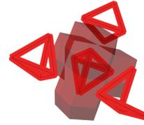
Figure 22: Idealization of tetrahedral brick units using tetrahedral beam cells, credit: RegoLight consortium, visualisation: Bollinger Grohmann, 2018
