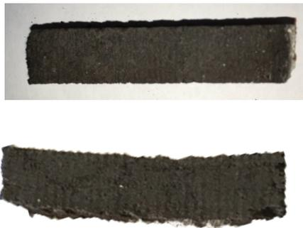
Figure 13: Samples 10 mm x 10 mm x 40 mm (top) and 10 mm x 20 mm x 70 mm (bottom) for bending tests, credit: RegoLight consortium, photo: DLR
