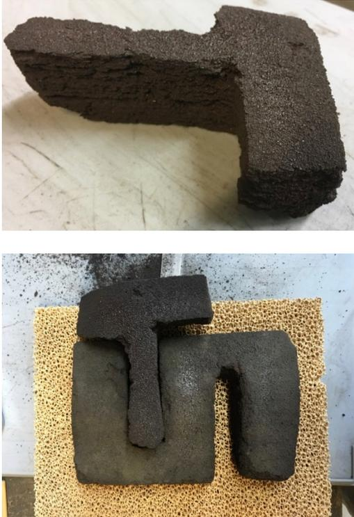
Figure 6: Solar 3D printed T-shape (top) interlocked in the S-shape (bottom), credit: RegoLight consortium, photo: DLR.
