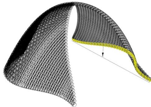
Fig. 5: Dome constructed from elements in Figure 4: with the centre of mass such that no scaffolding is needed, credit: RegoLight consortium, visualization: LIQUIFER Systems Group
