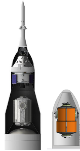
Fig. 1: I-HAB module in SLS ( left ) and SpaceX Falcon Heavy ( right ) payload shrouds. (© NASA/ ESA)
