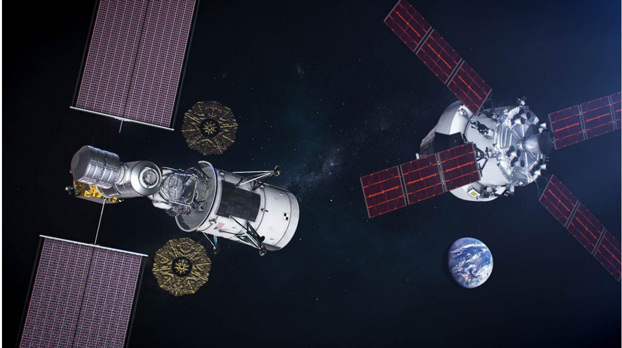
Fig. 1: The lunar orbital platform – GATEWAY: initial configuration to support ARTEMIS crewed lunar lander programme in 2024 (courtesy of NASA)
