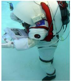
The Human Machine Interface also supports an advanced EVA Information System (EVAIS); a communication infrastructure involving CapCom, Mission Control in Brussels, external science centres, and prototype software allowing the astronaut to visualize procedures and communicate with Mission Control through either the chest-mounted tablet PC or the wrist-mounted control panel. Furthermore, Mission Control used the EVAIS to monitor the progress of the EVA (Extra-Vehicular Activity).
