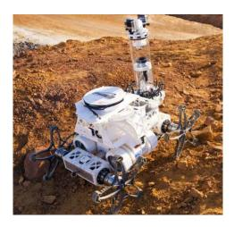
For use in the earth analogue simulations, YEMO was developed by the DFKI Robotics Innovation Centre in Bremen, Germany; a modified version of their ASGUARD design. As both a terrestrial (Mars) and an underwater (Moon) simulation were planned, a new amphibious robot was conceived.
