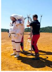
Mobile suitport: Steel frame for astronaut change in the field. Used to dock astronaut and release him/her from the weight of the suit at any time in case of emergency
