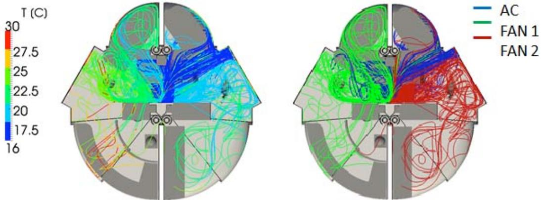
**Figure 9. Thermal Analysis – Streamlines colored by temperature (left picture) and streamlines colored by source (summer day in Death Valley); credit: SHEE Consortium, visualization: Sobriety, 2014**
