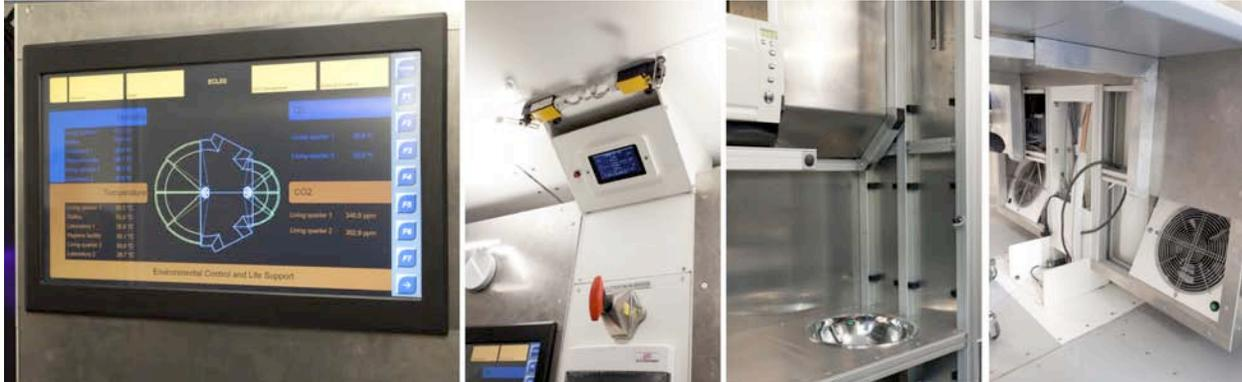
**Figure 6. SHEE control panel and unit, middle right: galley, far right: ventilation below the galley table;**
