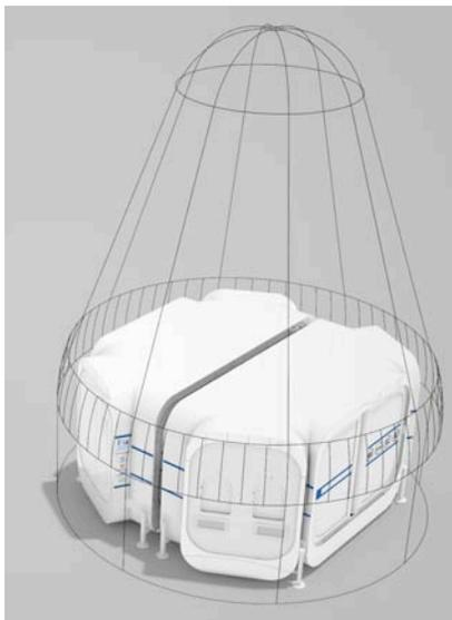
**Figure 1. Two stowed SHEE habitats fit into a heavy lift launcher with a diameter of 6m,**
