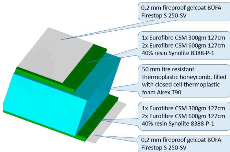
**Figure 3. Default wall composition and used materials, credit: SHEE Consortium, visualization: University of Tartu, 2014**
