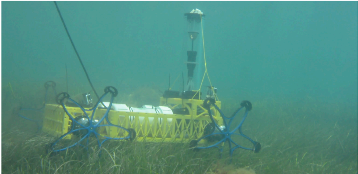
Figure 4. Test drive of the rover in 3m depth on a seaweed field. Credit: MOONWALK consortium, photo: Mathias Höckelmann, DFKI GmbH, 2015.
