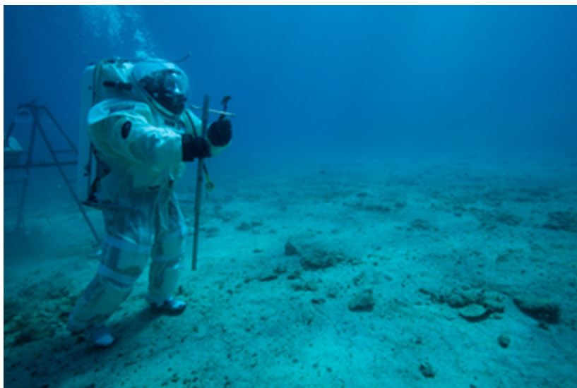
Figure 5. COMEX' GANDOLFI suit (1990 model) used for a lunar mission simulation at the sea bed offshore Marseilles (Frioul Islands); Photo courtesy A. Rosenfeld/COMEX
