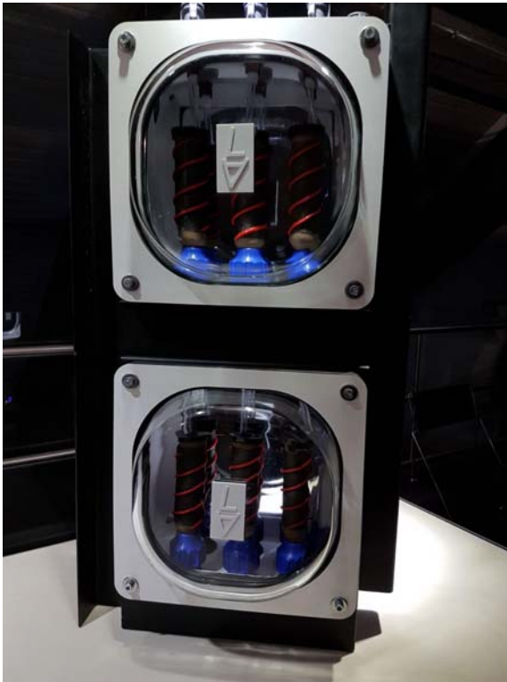
■ FIGURE 21.4 First test prototype 1 for a microbial fuel cell, vertically and horizontally stackable modular building element. Credit: Living architecture consortium, photo: LIQUIFER Systems Group, 2017.
