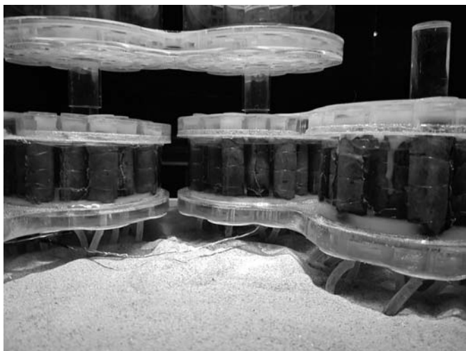
■ FIGURE 21.5 First test prototype 2 for a microbial fuel cell, indirect stackable modular building element. Credit: Living Architecture Consortium, photo: Simone Ferracina, University of Newcastle (2017).
