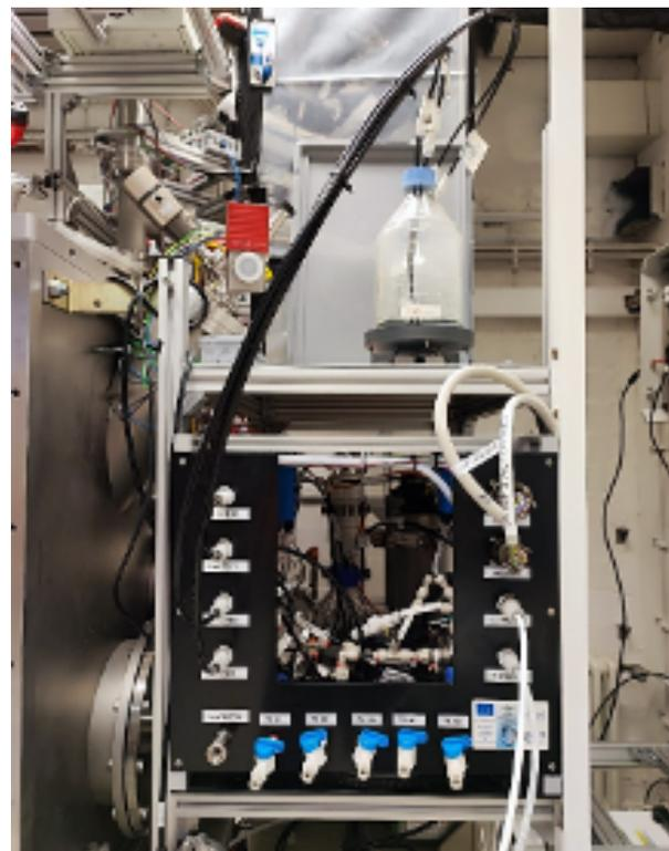
Fig. 4. WPS (black rack insert) integrated in a rack on the right-hand side of the TVAC. Storage II (glass bottles) on top of the rack.
