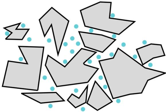
Fig. 8. A graphical representation of the unfused discrete icy-regolith. The high porosity of this specific sample means that even though ice is added, the thermal conductivity remains low.
