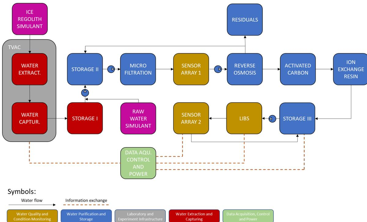
Fig. 1. System block diagram of all subsystems of the LUWEX experimental setup. Dashed arrows indicate signal interfaces. Solid arrows indicate water (solid, liquid or gaseous state) flow.
