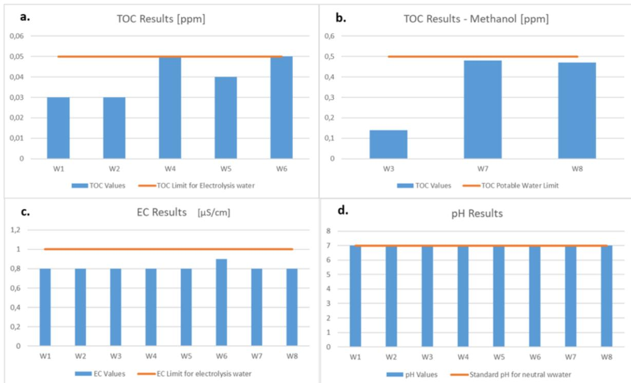
Fig. 5. Average TOC results for Ws without methanol, b. Average TOC result for Ws with methanol, c. Average EC results for all Ws, d. Average pH results for all Ws.
