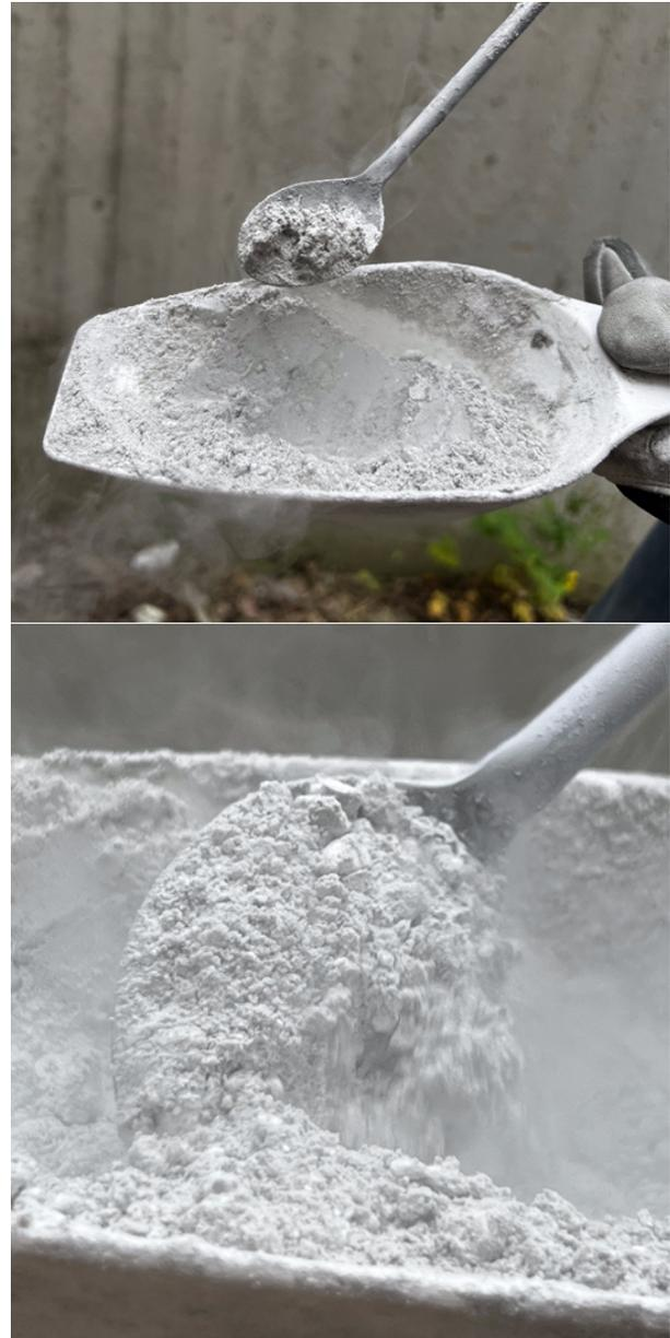
Fig. 7. The icy regolith simulant just after mixing in the ice particles. This process is done under cryogenic temperatures.
