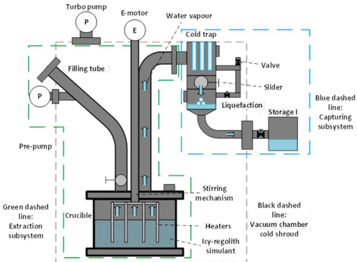
Fig. 2. Schematic overview of the WECS inside and partially outside the TVAC. The parts inside the green dashed line are the extraction subsystem, and the components encircled by the blue dashed line are the capturing subsystem.
