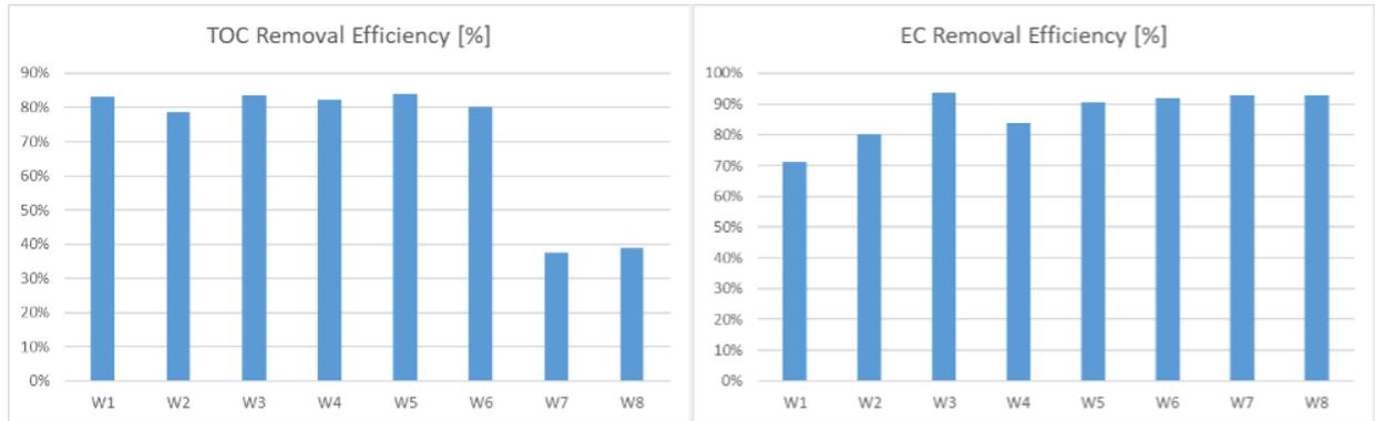
Fig. 6. TOC and EC removal efficiency calculated starting from the measurements of contaminants in inlet water.
