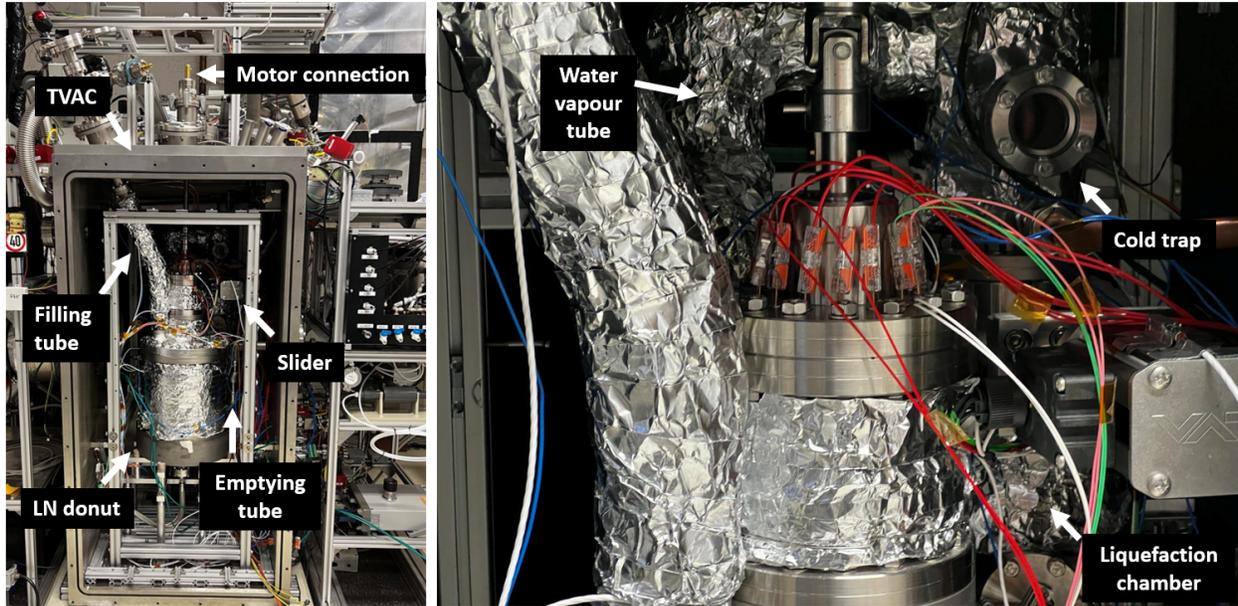
Fig. 3. Photos of the assembled WECS inside the TVAC.
