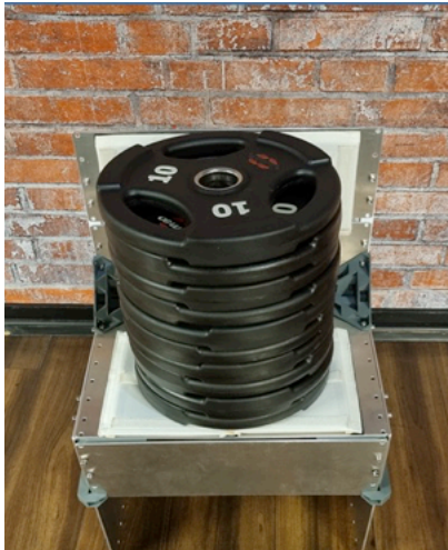
Fig. 10. Static load test of the demonstrator; [Source: LSG]
