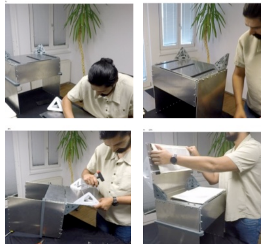
Fig. 12. Different pictures of the assembly procedure. Overall assembly time was 1.5h; Disassembly time was 0,5h. [Source: LSG]
