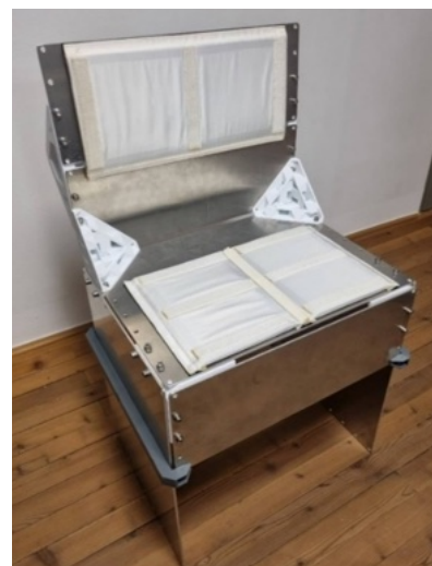
Fig. 9. Final manufactured and assembled chair (type one), including addition stabilization struts on the side of the chair. [Source: LSG]
