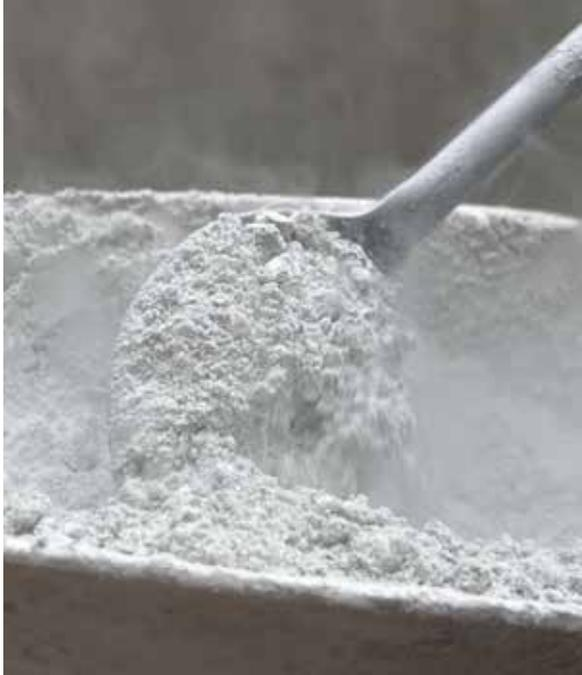
The icy regolith simulant just after mixing in the ice particles. This process is done under cryogenic temperatures.
