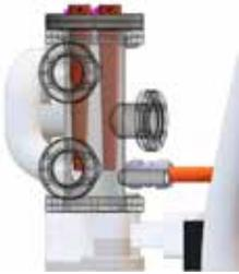
CAD drawing of the cold trap.
