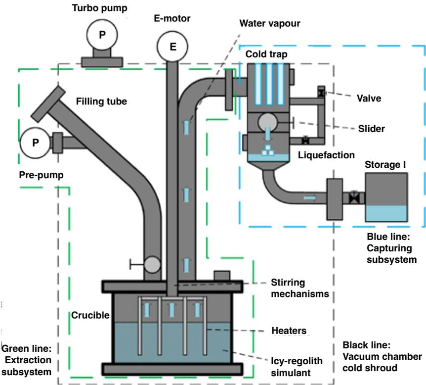
Top: Schematic overview of the WECS inside and partially outside the TVAC. The parts inside the green dashed line are the extraction subsystem, and the components encircled by the blue dashed line are the capturing subsystem.
