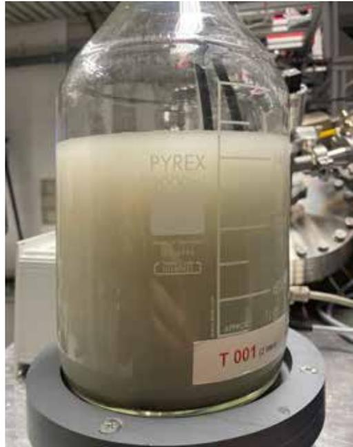
Polluted raw water directly after the water extraction and capturing process.
