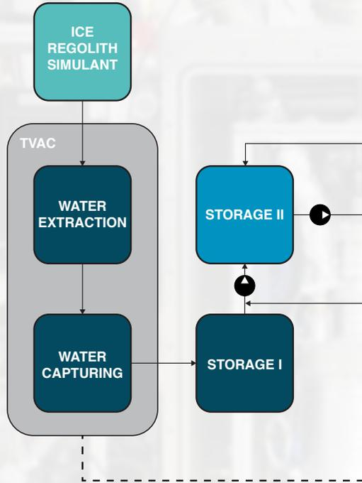
The figure above illustrates the material flow across the system. The extracted water is captured and stored in Storage I, a vacuum-rated tank connected to the TVAC. It is then transferred to Storage II, where its quantity is measured. The water is subsequently processed through purification stages, with quality continuously monitored. This integrated setup replicates the critical steps required for lunar water utilisation.
