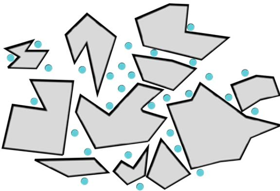
A graphical representation of the unfused discrete icy-regolith. The high porosity of this specific sample means that even though ice is added, the thermal conductivity remains low.
