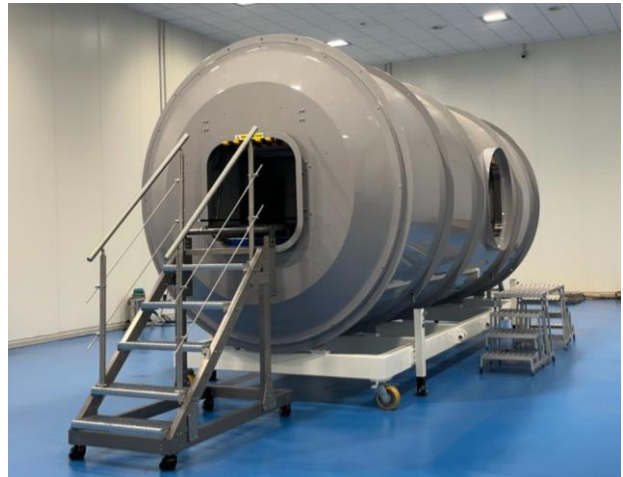
Fig. 4. Mock-up Primary Structure with stairs and support structure. (Copyright: Thales Alenia Space)
