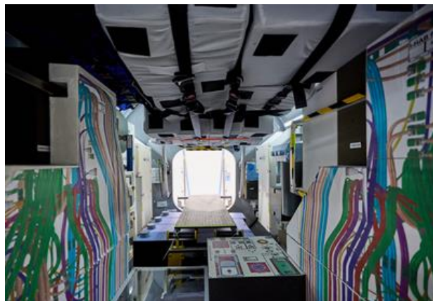
Fig. 7. LF Mock-up interior outfitting in cardboard, plastic and foam
