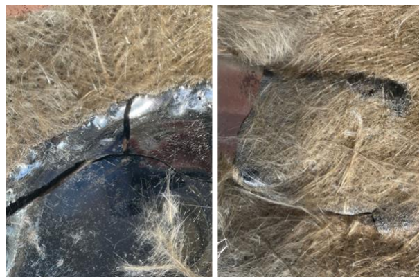
Fig. 11. Casting onto woven fibers. Close-up of a sample produced during the printing campaign: Fibre-cast part: top view (left) and bottom view (right).
