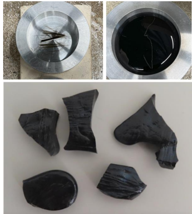
Fig. 5. Casting onto single fibers strategy. Samples produced during the printing campaign.
