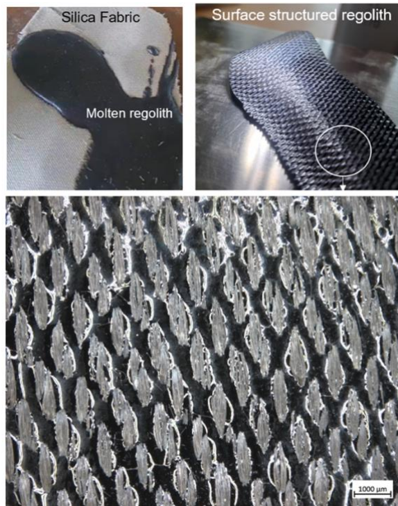
Fig. 13. Fiber-imprinted casting. Sample produced during the printing campaign, with a close-up on the surface pattern.
