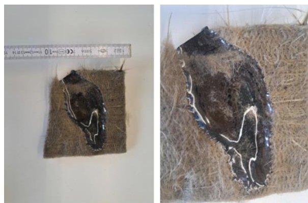
Fig. 10. Casting onto woven fibers. Sample produced during the printing campaign.
