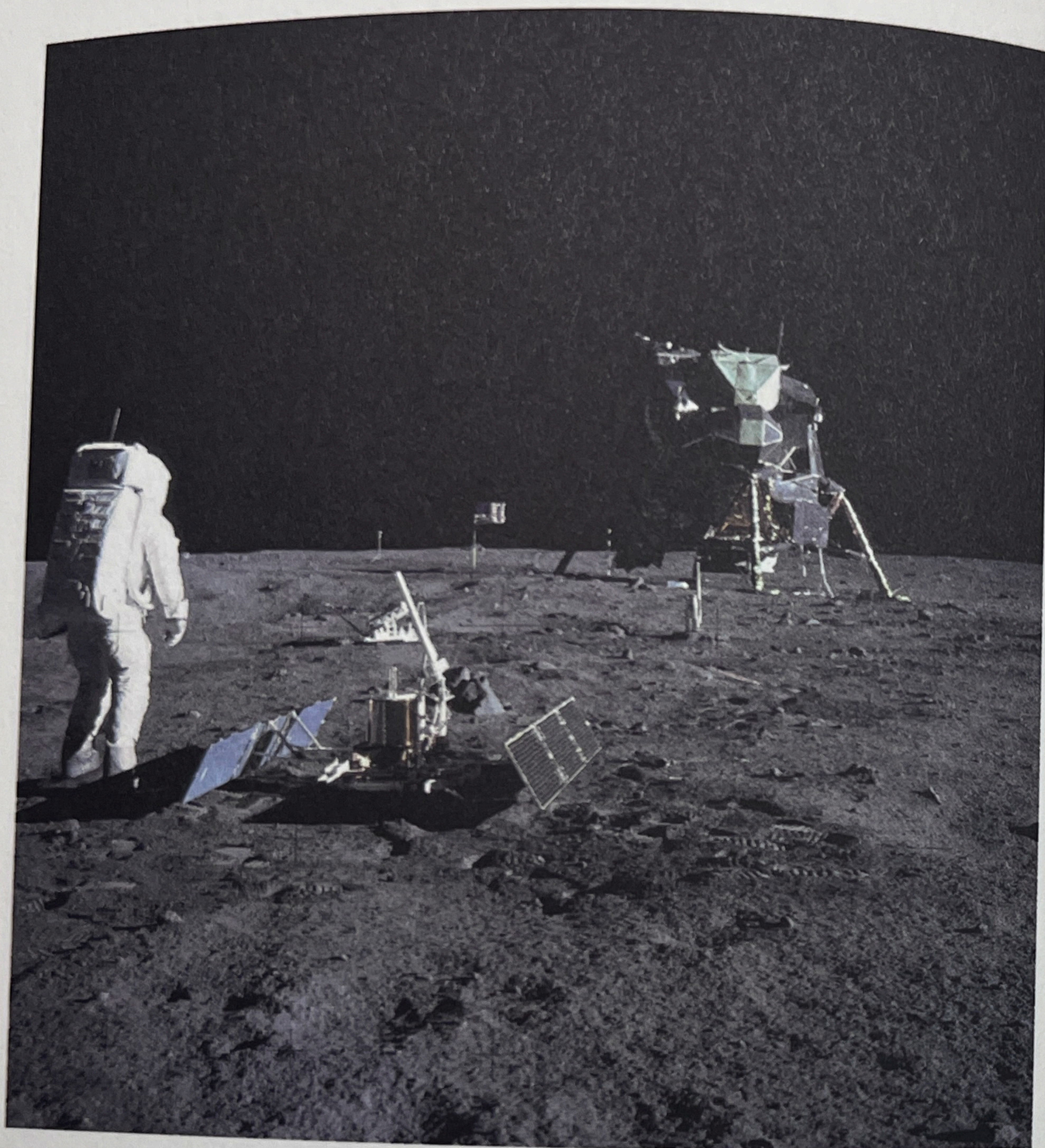
Abb. 2: Aldrin Gazes at Tranquility Base during the Apollo 11 extravehicular activity on the moon. He had just deployed the Early Apollo Scientific Experiments Package. In the foreground is the Passive Seismic Experiment Package; beyond it is the Laser Ranging Retro-Reflector (LR-3). Courtesy of NASA.
